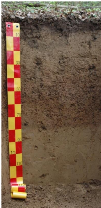
Figure 8.5: Ideal soil profile. Always take the photo perpendicular to the profile wall
